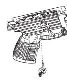
翻轉至另一側將選擇鈕卸下 Disassemble the Fire Selector on the opposite side
