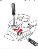
3 旋轉覘孔調整覘孔高度。 Rotate the sight drum to adjust the height of the sight.
