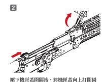
定在前。(需確實向前固定避免落下夾傷) Press the upper receiver catch to open the remove the charging handle set. upper receiver cover and keep it opening in the front. (Avoid the upper receiver falling from hands clipping)
