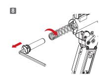
使用5mm六角扳手,將尾頂桿向內壓入轉至 45度即可將尾頂桿與彈簧一同抽出。 Use 4mm Allen Key, insert it to the spring guide and then press down to turn 45 degrees then take out the spring guide and spring.
