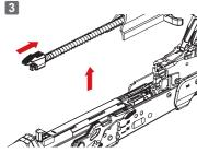
將機匣蓋開關向前推取出槍機拉柄組 Push the upper receiver catch forward to
