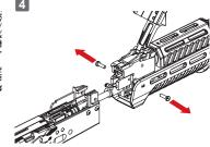
將槍管座螺絲卸下,並將槍身前段往前抽出。 Remove the barrel mount screws, and then pull the front assembly forward to remove.
