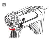
將槍托摺疊後,把線材抽出槍托。 Fold the stock and then and unplug
