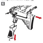
將握把與射擊選擇桿卸下。 Remove the Ergo grip and the fire selector Remove the gearbox upward to separate
