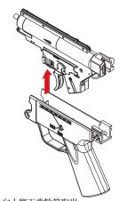
向上將下齒輪箱取出 Remove the lower gearbox by pulling it upward.
