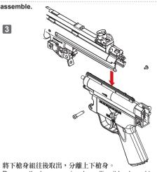
Remove the lower receiver by pulling it backward to separate the upper and lower receivers..
