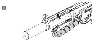
將電池接頭固定好後,再把護木固定至定位。 Plug in the battery, then reassemble the handguard and the pin.
