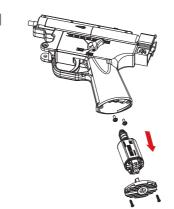
旋開馬達底蓋螺絲,將馬達底蓋及馬達卸下。 Unscrew and remove both motor butt plate and the motor.
