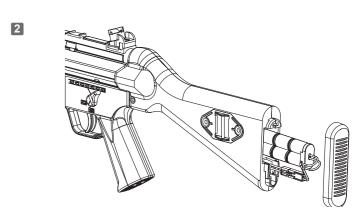
將電池接頭固定好後放入槍托內,再把槍托底板固定至定位。 Plug in the battery, put the battery into the stock, and reassemble the butt plate.
