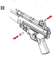
將前槍身結合銷旋開取下。 Remove the front receiver pin.
