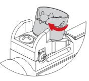
4 調整完畢後再將螺絲鎖緊。 Screw the fixing screw to fix after you finish adjusting.
