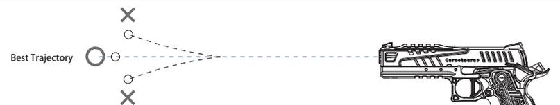
H-up Adjustment: Make sure the trajectory of the BB pellets to be straight. Rotate the screw clockwise to raise the trajectory. Rotate the screw counterclockwise to lower the trajectory.
